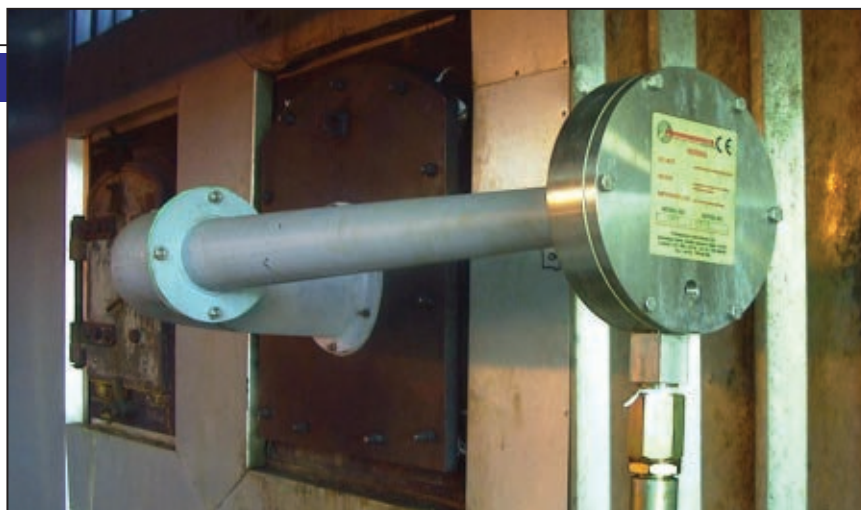
FIGURE 4. AACs are non-intrusive, and can be employed wherever dry materials are processed, generated, stored or transported. A periodic “sounding” (typically 5–10 s every 10–60 min) is all that is required to achieve the desired goal
