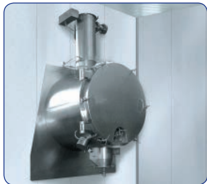
Italvacuum's PLANEX System installed through the wall of a clean room
