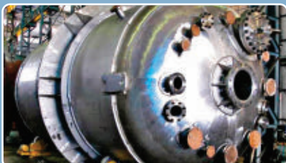
Alloy-20 Reaction-cum-Filtration Vessel
