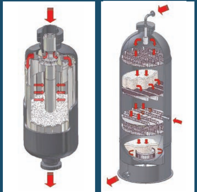
Radial Flow and Down Flow reactor internals
